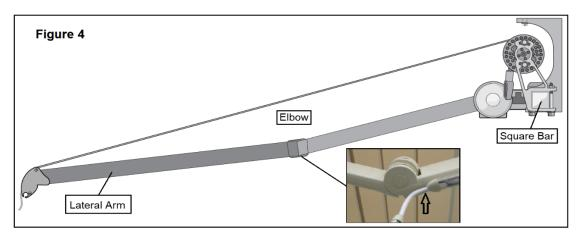
7. When the LED Segment is centered on the arm, press firmly along the tape strips to set themin place. Wrap the power cord behind the square bar on the awning.
